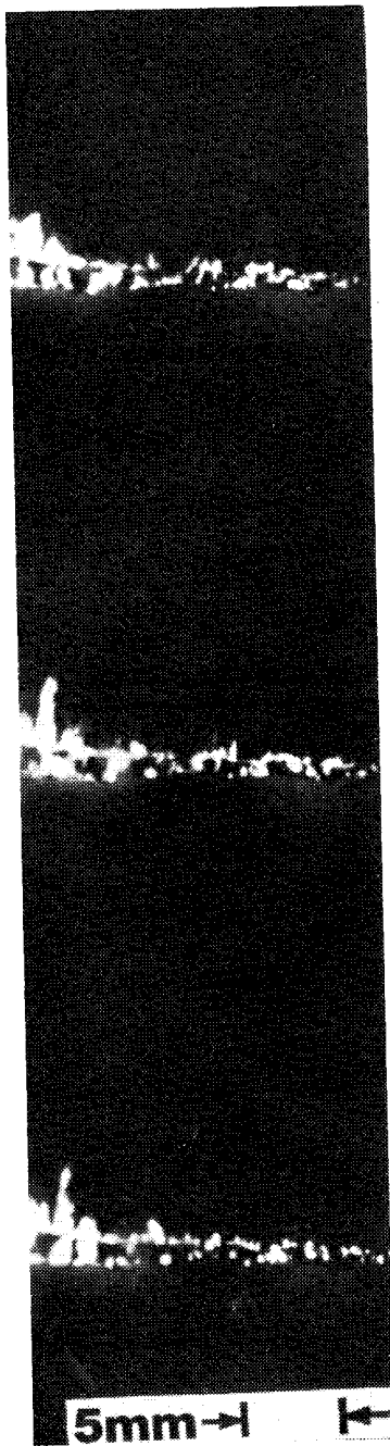
Fig. 4 Diffusion flamelets associated with the AP-binder interfaces. Successive frames from motion picture, 0.001 s between pictures. Total sample width 2 cm: HTPB binder, tapered from 130 \mu\text{m} (left) to 10 \mu\text{m} . Pressure 6.9 MPa (1000 psi).
